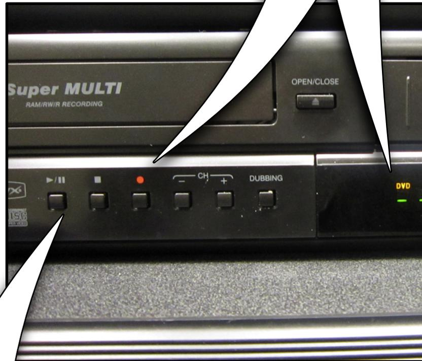
If you want to finish the recording before the end of the tape, press PAUSE on the JVC player, and then STOP on the MiniDV tape
